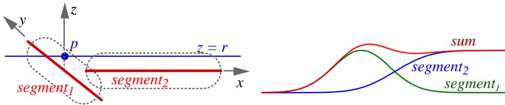
**Figure 5.65 ‘Tee’ Junction with Left Endpoint of Segment<sub>2</sub> Moved Amount  $r$**
