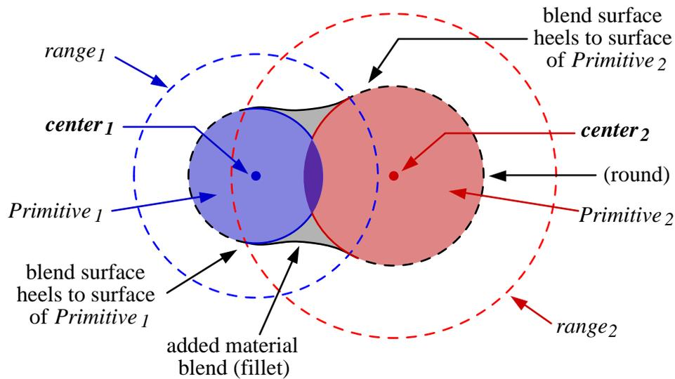
**Figure 5.26 The Elliptic Blend**
