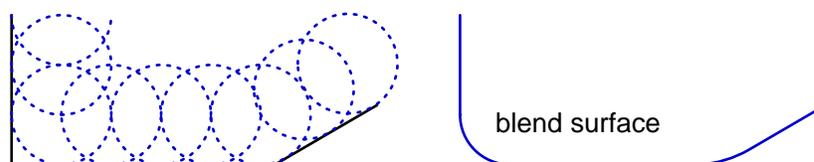
**Figure 5.23 The Rolling Ball Blend**
