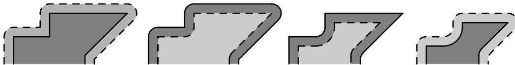
**Figure 5.24 Approximation to the Rolling Ball Blend**
