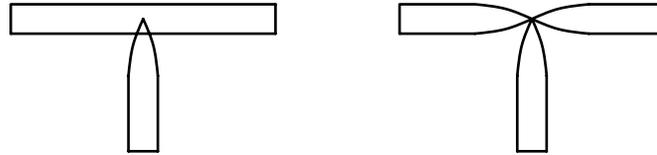
**Figure 5.69** *Two Methods of Tapered Junction*
