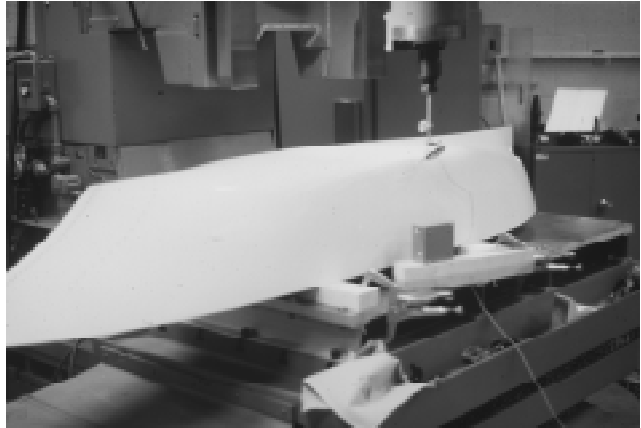
Fig. 6. The milling machine being used as a digitizer.
